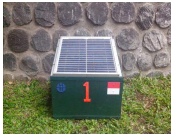
Gambar 6. Unit Automatic Boundary Marker .
