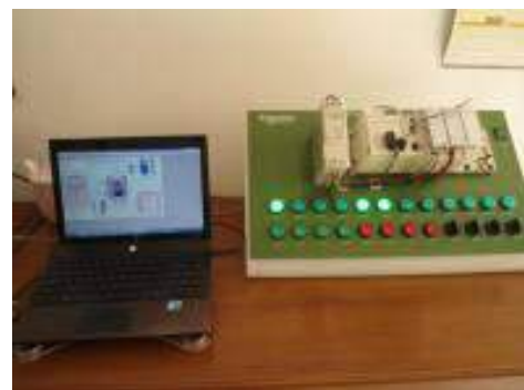
Gambar 7. Tampilan SCADA + PLC
